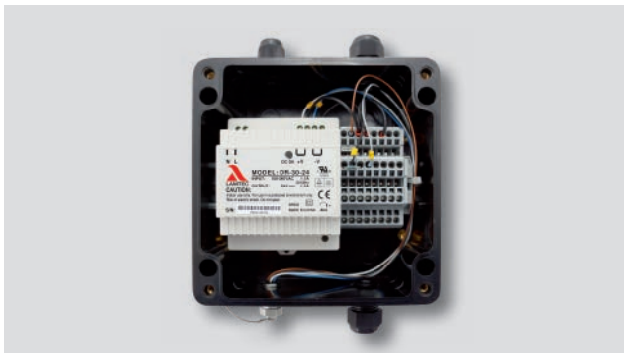
FN30-10 in the connection housing with FSB plug connector.
